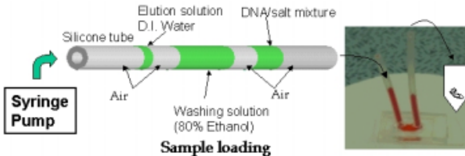
Fig. 7. Test bench of DNA purification chip.
